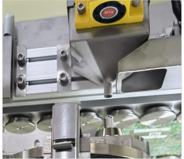
12. Standard with the nozzle automatic cleaning function, Strong cleaning of nozzles with cleaning powder.
