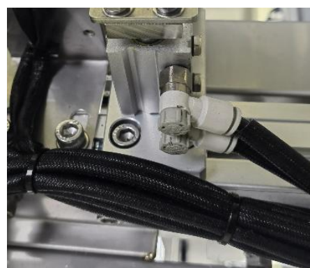
Additional protection of all access lines
