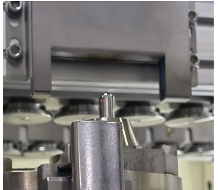
14. Laser detection system for soldering wave height (option).
