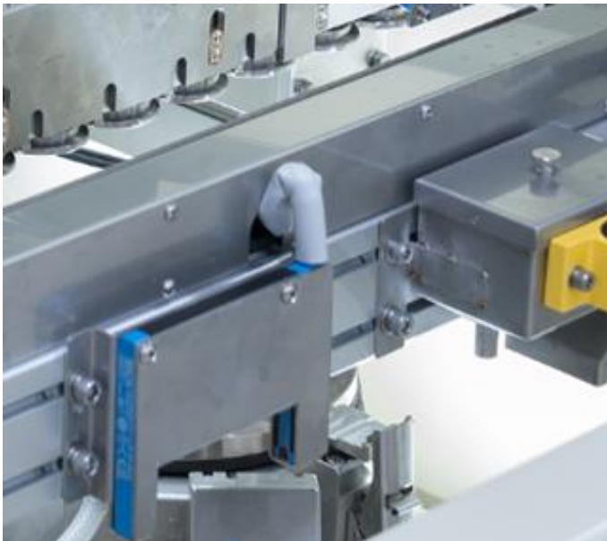
14. Laser detection system for soldering wave height (option).
